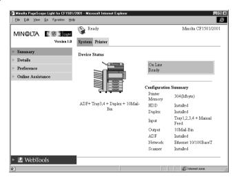
**Device Status** This area uses graphics and text to shows the configuration of options installed on the CF1501/2001.
